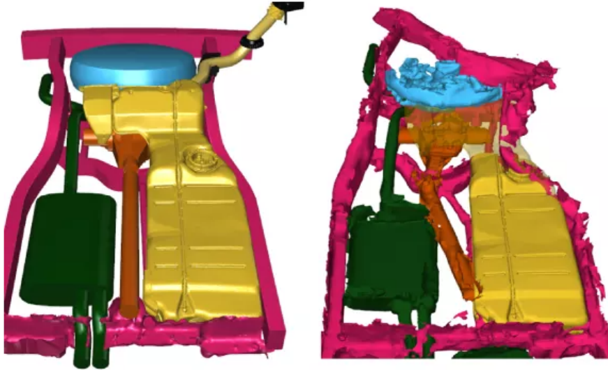
Figure 1: Finite element model showing chassis components during impact
